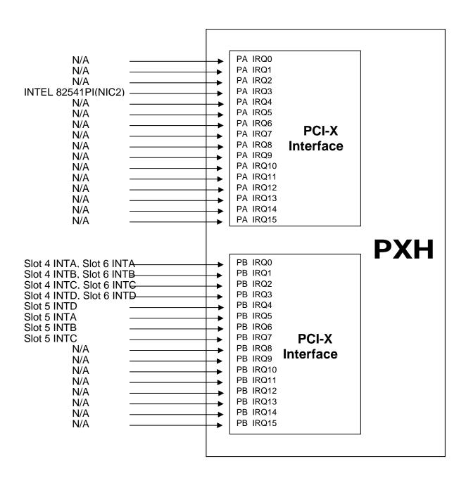
Figure 5. PXH Interrupt Routing Diagram
